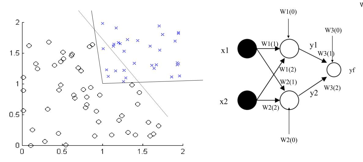
The propagation pass begins at the first hidden layer by presenting it with the input vector, and terminates at the output layer by computing the output signal for each output neuron
